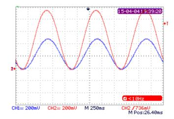
Sinusodial control signal; P1 set to 500mA/V; red: signal at V.C. input; blue: load current, 1mA/mV
