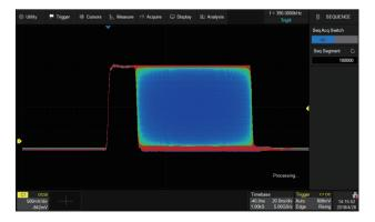
Segmented memory collection will store the waveform into multiple memory segments (up to 100,000) and each segment will store a triggered waveform as well the dead time information. The interval between segments can be as small as 2  $\mu$ s. All of the segments can be played back using the History function
