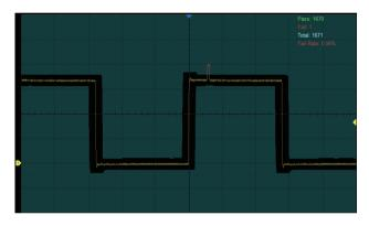
Hardware-based High Speed Mask Test Function
