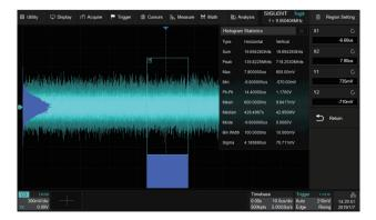
The Waveform Histogram feature provides a statistics view of the waveform in horizontal and vertical directions
