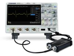
the SDS5000X can control the SAG1021I USB Function/Arbitrary waveform generator to output waveform with up to 25 MHz frequency and  $\pm 3$  V amplitude. Six basic waveforms plus multiple types of arbitrary waveforms are built-in
